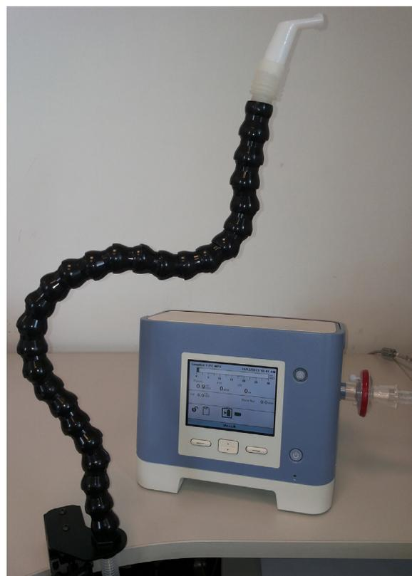
Figure 2 Open mouthpiece ventilation dedicated circuit.
